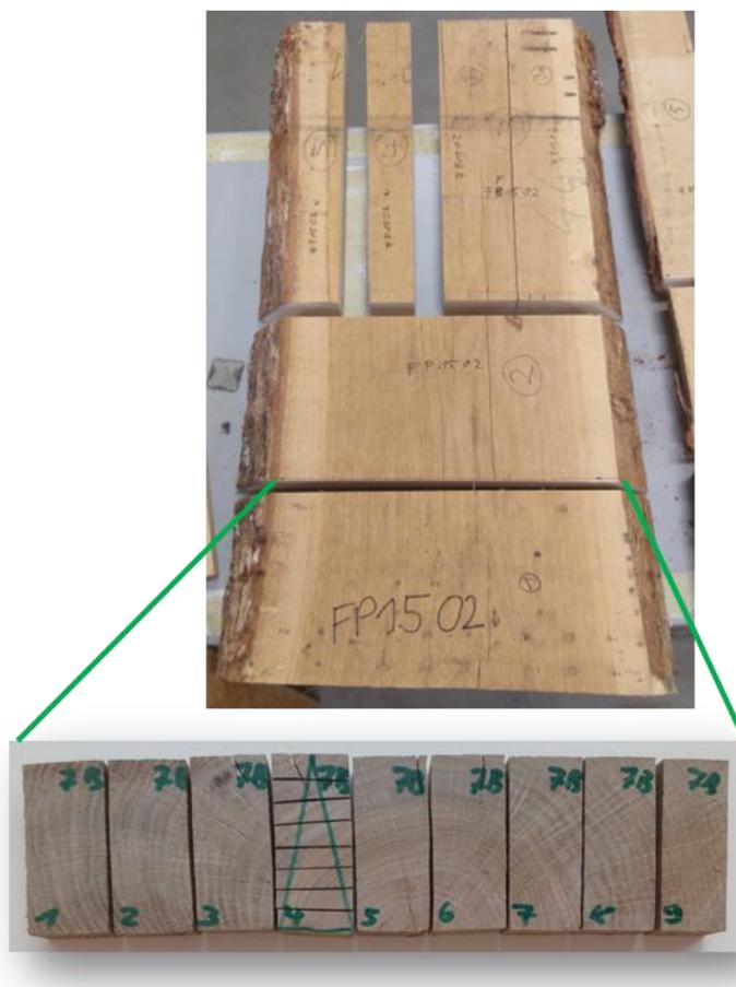
*Figure 2: Sample preparation for “cloud”- investigation and wood moisture determination*
