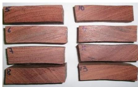
Figure 5: Jarrah board cross sections after MW drying
