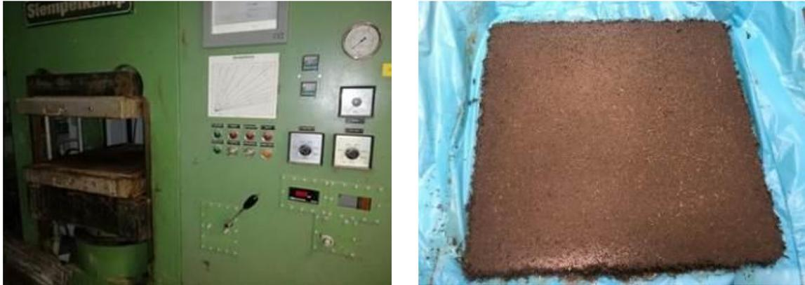
Figure 1: Seimpelkamp press, CBPB after 24 hour of pressing (right)
