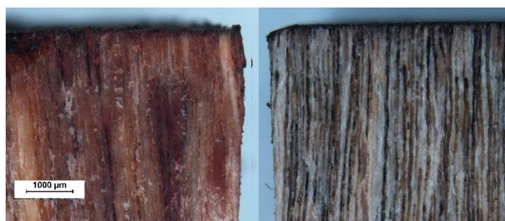
*Figure 4: Comparison of KSCN stained (left) and unstained (right) beechwood with magnetite*
