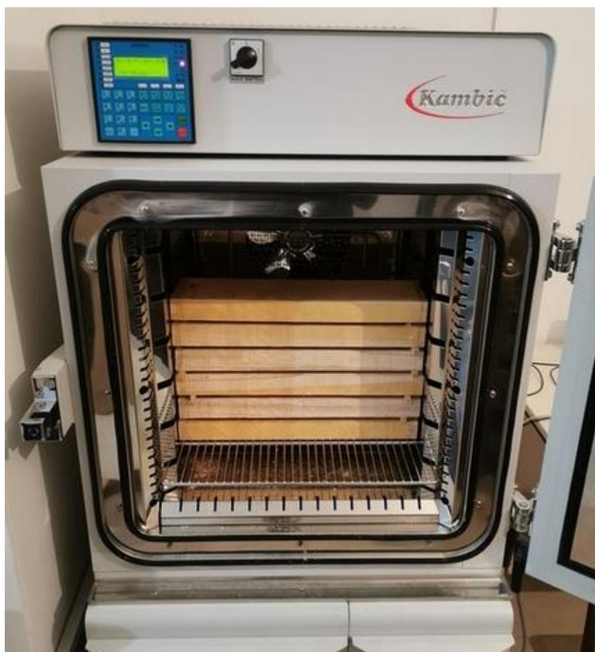
*Figure 1: Climatic chamber with beech boards*
