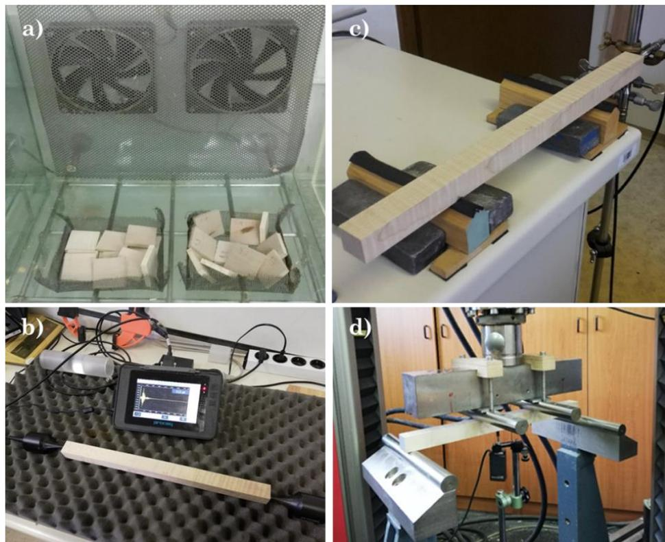
**Figure 15: Determination of dimensional stability (a), ultrasound velocity and moduli of elasticity (b), vibration damping (c) and static bending strength (d) of straight grained and wavy sycamore maple**
