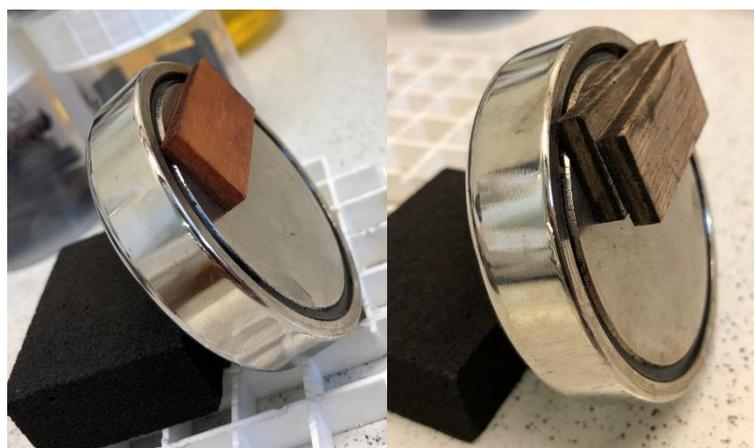
**Figure 5: poplar and linseed oil-based magnetite system (left), tannin-based magnetite system (right)**
