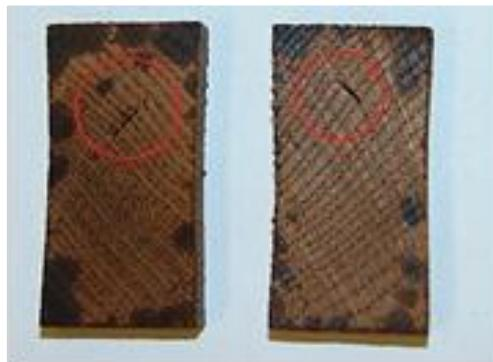
**Figure 2: Radial cracks and deformations on the cross section of *Ailanthus* (source: Bak and Németh 2015)**
