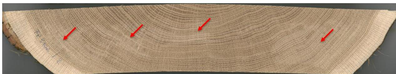
*Figure 1: Typical “white clouds” (arrows) surrounded by darker colour at the edges of the cross-section*
