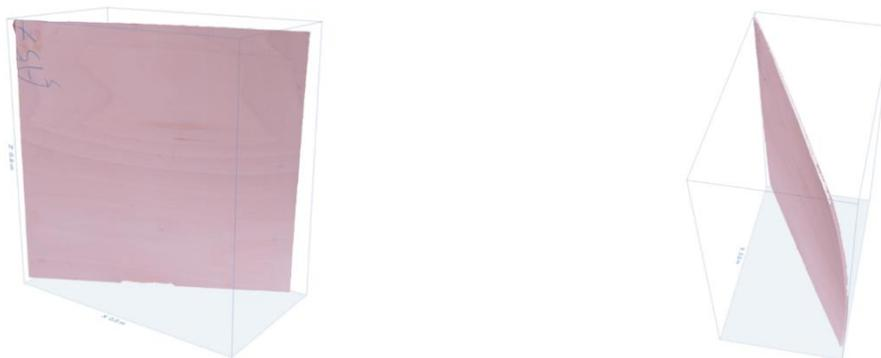
**Figure 2: 3D model of a plywood panel obtain by photogrammetry method**
