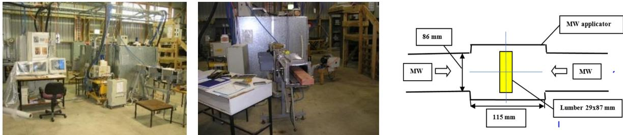
Figure 1: MW conveyor plant for timber modification 2x30 kW (frequency 2.45 GHz) and board position in 2 port MW Applicator (115x115x350 mm)
