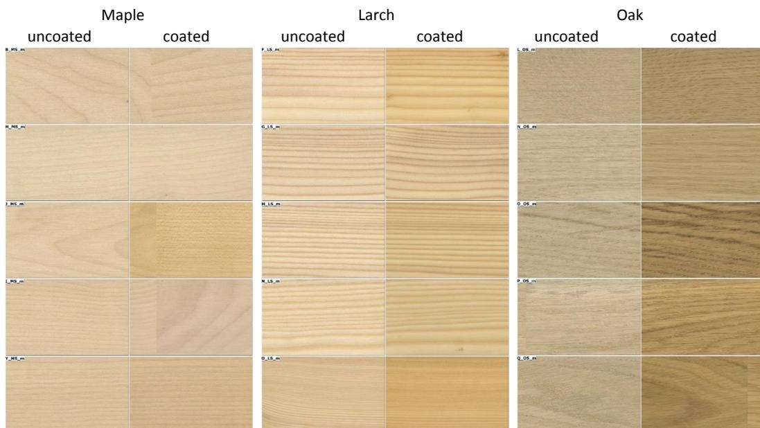
*Figure 1: Scans of uncoated and coated wooden floors with maple, larch and oak top layer*
