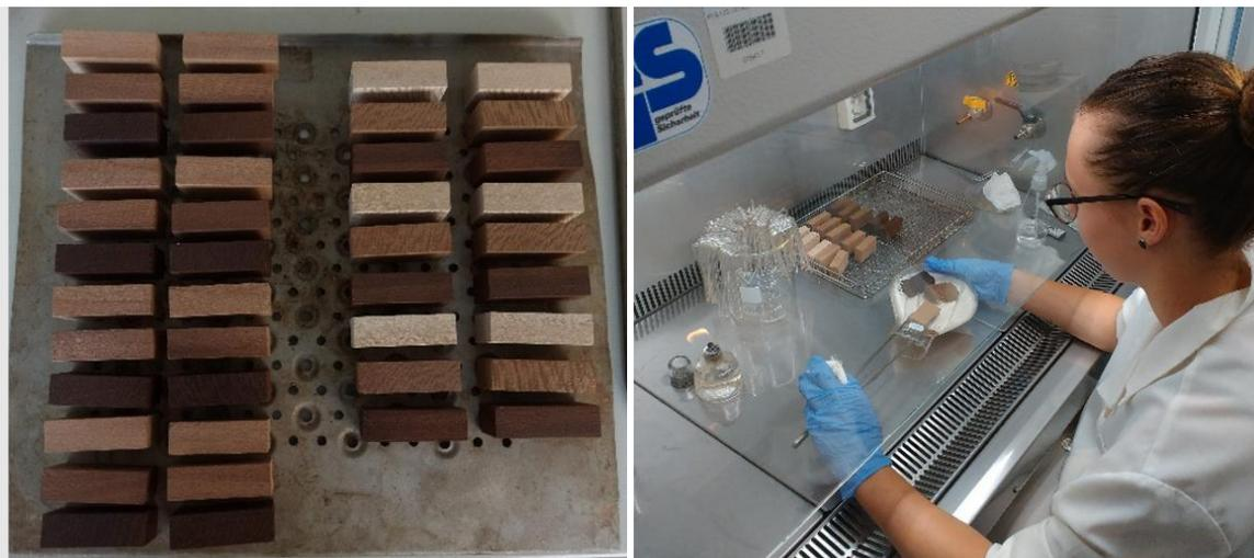
*Figure 2: Specimens (left), and placing of specimens into Kolle-flasks (right)*
