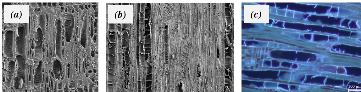
Figure 1: Scanning electron micrograph of (a) wound-wood and (b) reaction zone (FEI Quanta SEM, mag. of 1000 x and 353 x ). (c) Autofluorescence of tyloses in the vessels of reaction zone (OVEN ET AL. 2010).
