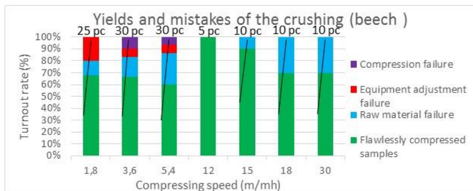
Figure 2: Yields and the mistakes during the beech samples crushing in the 1st experiment suite ( 1,8 - 5,4 \frac{m}{m \cdot h} ) and in the 2nd experiment suite ( 12 - 30 \frac{m}{m \cdot h} )
