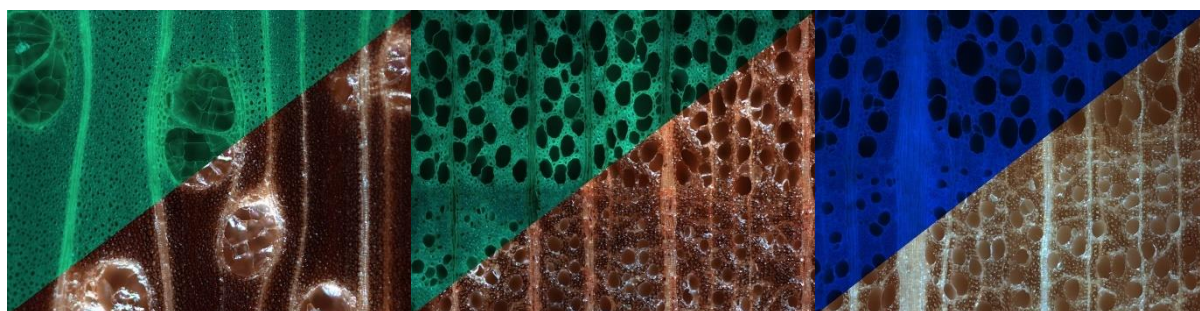
Figure 1: UV-detection of robinetin-derivative (indicated by green colour) in 70yr-old Robinia (left) and robinetin-impregnated beech wood (middle) compared to robinetin free beech wood (right; indicated by blue colour) in upper-left halves of microscopic photos; lower-right halves: without UV-detection in normal light
