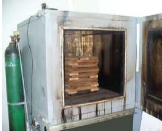
Figure 1: Experimental heat treatment chamber
