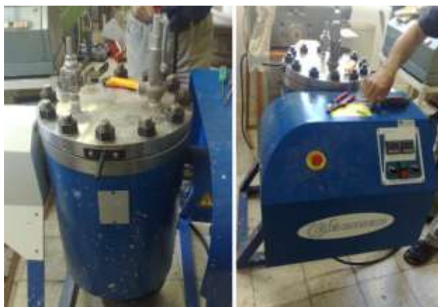
Figure 6: Reactor for acetylation
