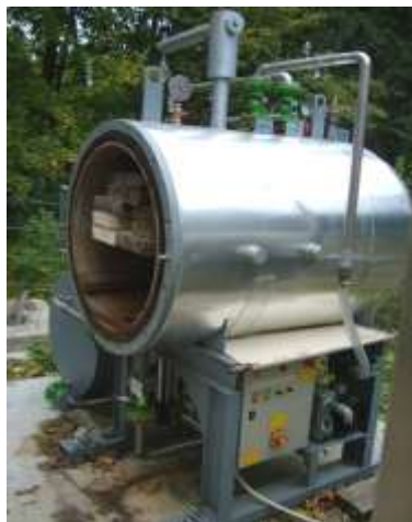
Figure 2: Combined treatment autoclave
