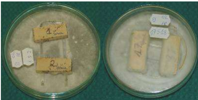
Figure 8: Anti-fungal effect of nanozinc (left: treated; right: untreated)
