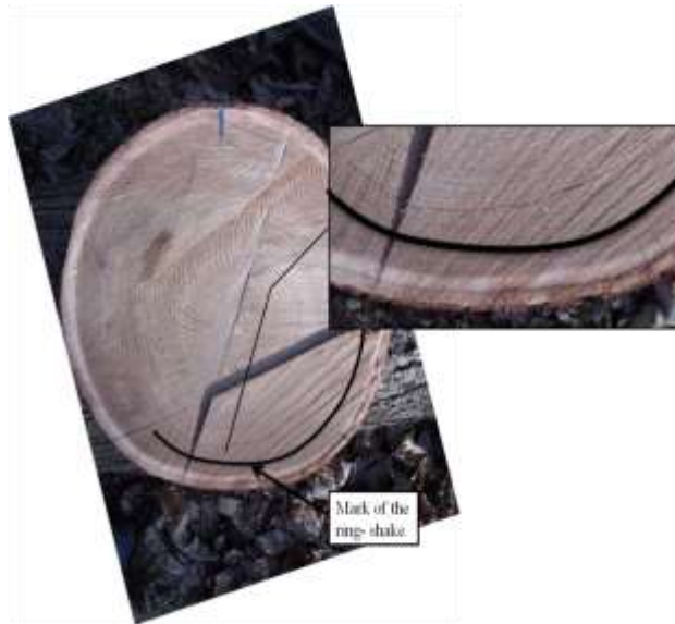
Figure 4: Principal of drawing ring-shake in the tomographs
