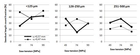
Figure 2: Count fractions of sawdust length (<125  $\mu$ m, 126-250  $\mu$ m and 251- 500  $\mu$ m) with variable saw tension for saw set s1=0,57 mm and s2=0,47 mm
