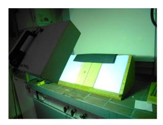
Figure 1: The quartz lamp of VT-800 type and samples under exposure
