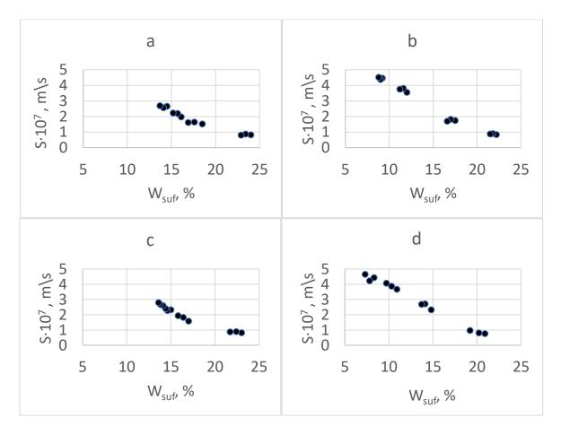
Figure 1: Effect of surface moisture content (Wsuf) on the mass transfer coefficient (S) at different values of temperature (t) and relative humidity ( $\varphi$ ) of air ( $a - t = 50^{\circ}$ C,  $\varphi = 73\%$ ;  $b - t = 50^{\circ}$ C,  $\varphi = 45\%$ ;  $c - t = 60^{\circ}$ C,  $\varphi = 73\%$ ;  $d - t = 60^{\circ}$ C,  $\varphi = 45\%$ )
