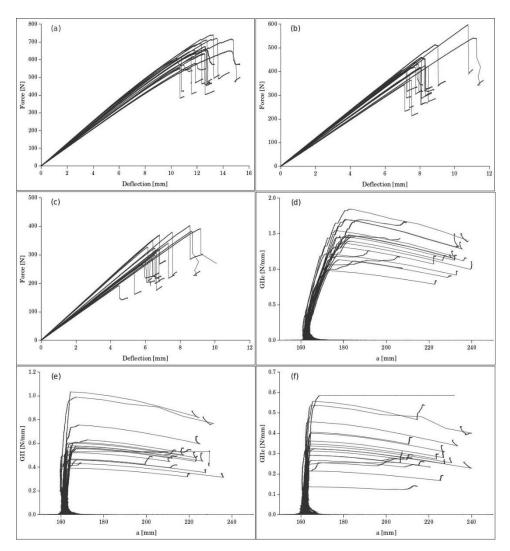
Figure 4: Force-deflection curves for: (a) non-treated wood, (b) treated at  $180 \, ^{\circ}\text{C}$ , (c) treated at  $200 \, ^{\circ}\text{C}$ ; Energy release rate dependent on equivalent crack length of: (d) non-treated wood, (e) wood treated at  $180 \, ^{\circ}\text{C}$ , (f) treated at  $200 \, ^{\circ}\text{C}$
