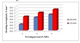
Fig. 1. Relationship between the bending strength of FBs and the pressing pressure and PFR content
