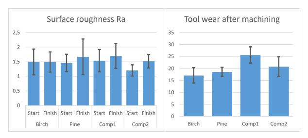
Figure 1. Change in surface roughness and tool wear in machining.
