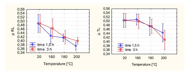
Fig. 2 Poisson's ratios µRL and µTL after thermal treatments. Bars stand for 95% confidential limit.
