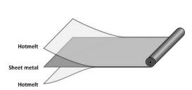
Figure 1. Structure of a pre-coated electric heatable composite adhesive tape (© Fraunhofer WKI)
