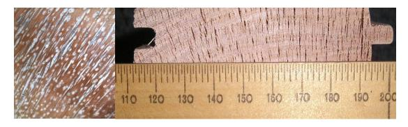
Figure 1. Blue gum wood cross cut (left) after Moderate degree MW modification. Narrow white lines are original rays, wider white lines are ruptured rays. Mountain Ash (right) wood structure after High degree MW modification.
