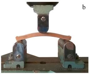
Figure 1: Specimens compressed in a mould (a) and specimen in testing device before bending strength test (b)
