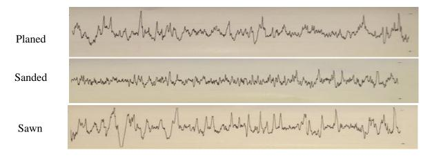
Figure 1: Surface roughness profile of poplar for planed, sanded and sawn surfaces.
