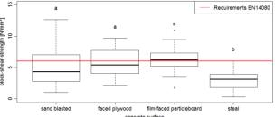
Figure 3. Block-shear-strength acc. to EN 14080 on beech wood for cold-curing process
