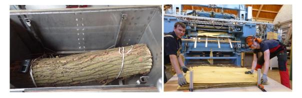
Figure 1: A Robinia log in the cooking unit (left) and the new RAUTE peeling machine at the WKI (right)
