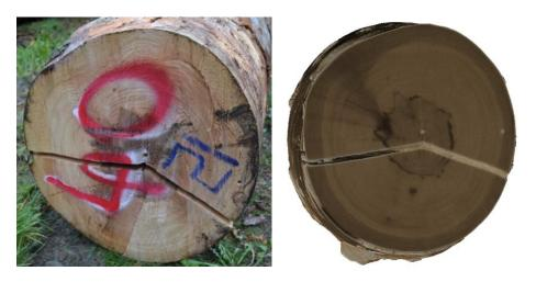
Figure 3: Comparison of wood characteristics within a beech log (left: photo, right: CT-image) ©MiCROTEC
