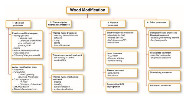
Figure 1: A diagram of the various wood modification processes
