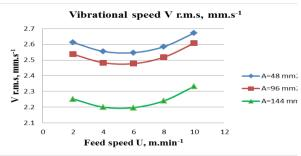
Fig. 3. Vibration speed measured at a point Ax
