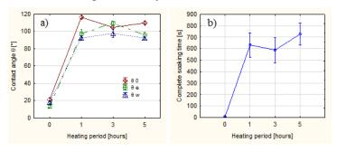
Fig. 1 Duration of heat exposure of beech wood at 200 °C affecting the contact angle values (a) and the time necessary for complete soaking of the drop into the wood substrate (b).
