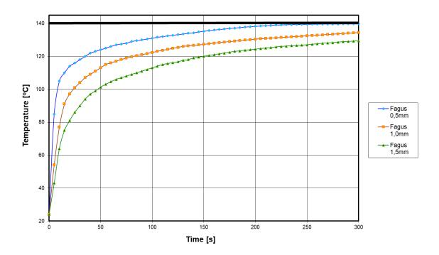
Figure 1. Change of the border temperature chipboard - veneer, at  $T = 140^{\circ}C$
