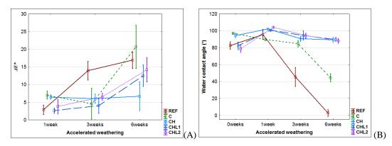
Figure 2: Colour (A) and surface wetting (B) changes of coated oak wood during accelerated weathering
