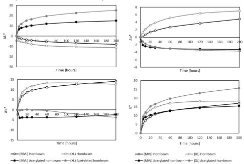
Figure 1: Change of colour coordinates ( $L^*$  - lightness,  $a^*$  - red hue,  $b^*$  - yellow hue) and total colour change ( $E^*$ ) of untreated and acetylated hornbeam irradiated by mercury-vapour lamp (MVL) and xenon lamp (XL) for 200 hours
