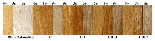
Figure 3: Visual changes of oak wood with different coatings during 6 weeks of accelerated weathering
