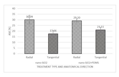
Figure 1: ASE of nano-silica treatments on beech wood (whiskers showing standard deviation of the results)
