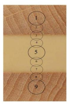
Figure 3 Model of wood bonding representing the bulk material (1, 5, 9), interface (3,7) and the interphase region (2, 4, 6 and 8) according to Marra et al. (1980)
