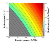
Fig. 2. Lines of constant levels for bending strength in case of super hard FBs with increased load-carrying capacity
