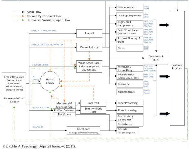
Figure 1: Various hardwood process chains including side streams indicating the most dominant species per chain (short code for single wood species according to EN 13556), not fully elaborated
