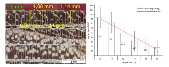
Figure 2: Measurement of the lathe checks depths (left) and the correlation between the medium depths and the cooking temperature of the black locust log.
