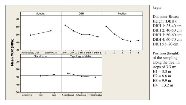
Figure 1: Main forest and harvest parameters effects on the mean bending strength (Mean MOR) of French
