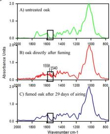
Figure 1: Spectral range at 2000 to 800 cm<sup>-1</sup>, with focus on the affected area (1575 – 1535 cm<sup>-1</sup>), where A) shows untreated oak, B) oak directly after fuming, showing the signals (1558 and 1540 cm<sup>-1</sup>) related to the fuming process and C) after 29 days of airing
