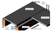
Figure 2. Timber-concrete joints by electrical heated adhesive tapes (© IFS-TU-Braunschweig)
